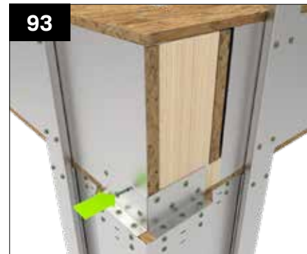
93 On corners, fit the clips to the beam as per the walls. Fit the 2 additional corner angle brackets WPPF001 to each side as shown using GPHS050 screws.
