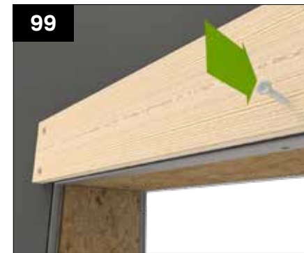
99 Above openings, fit a horizontal batten across the top of the opening at 450mm centres with the base of the batten aligned with the opening in the wall.
