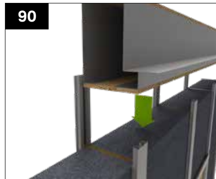
90 Lower the Flat Roof beam into position onto walling panels, the clips will run up both the internal and external face of the Flat Roof beam.
