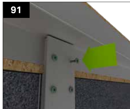
91 Once the beam is in position fix in place using the provided GPHS fixings into the beam with two fixings and the walling panels with two fixings for every full clip.
