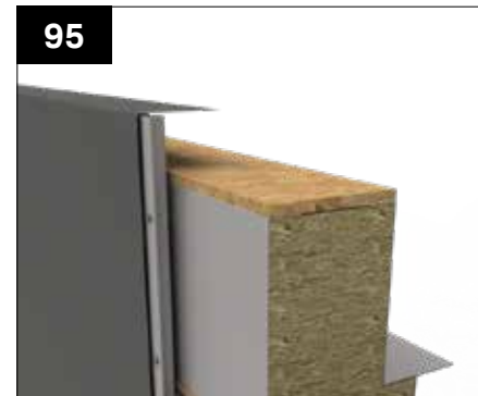
95 When applying the membrane this is to be folded over at the top of the clips as shown above.
