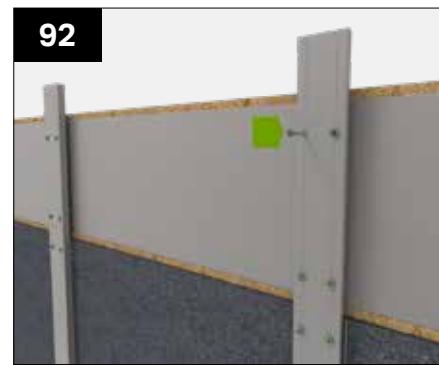
92 Externally secure each walling clip into the beam as shown using two GPHS fixings 30mm from the top and bottom of the beam and two fixings into the walling panels.
