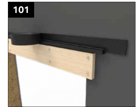
101 Using tape provided seal along the joint at the top between the soaker trim and the membrane.
